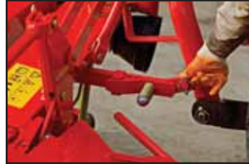
Figure 8- Connect the tension pin and control (2)
