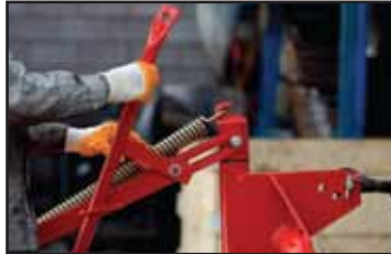
Figure 7- Disconnect the tension spring (1)
