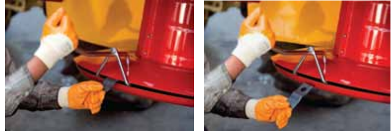
Figure 17- Replacing the knives
